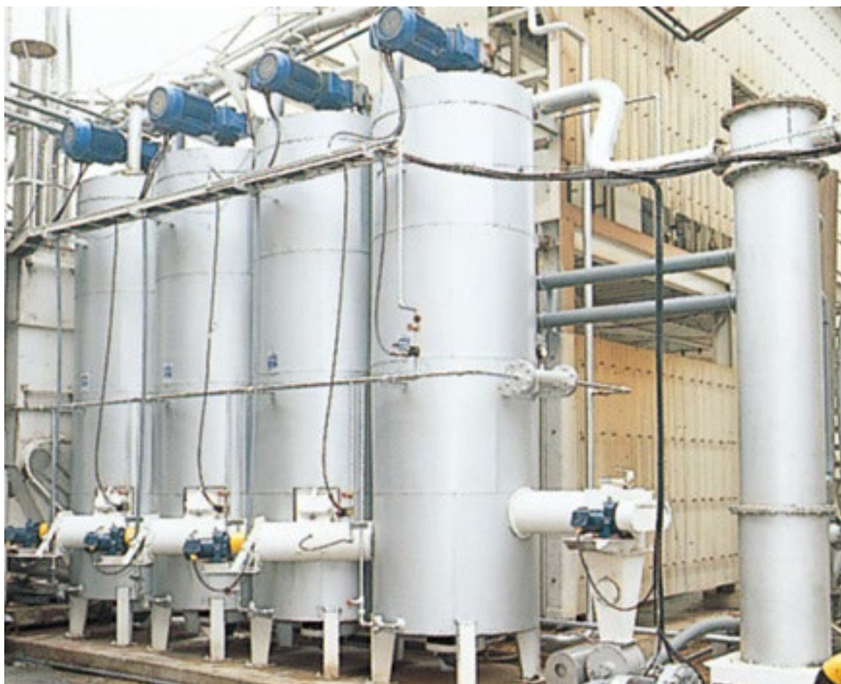
A cyclone dryer installed at a food processing manufacturer
